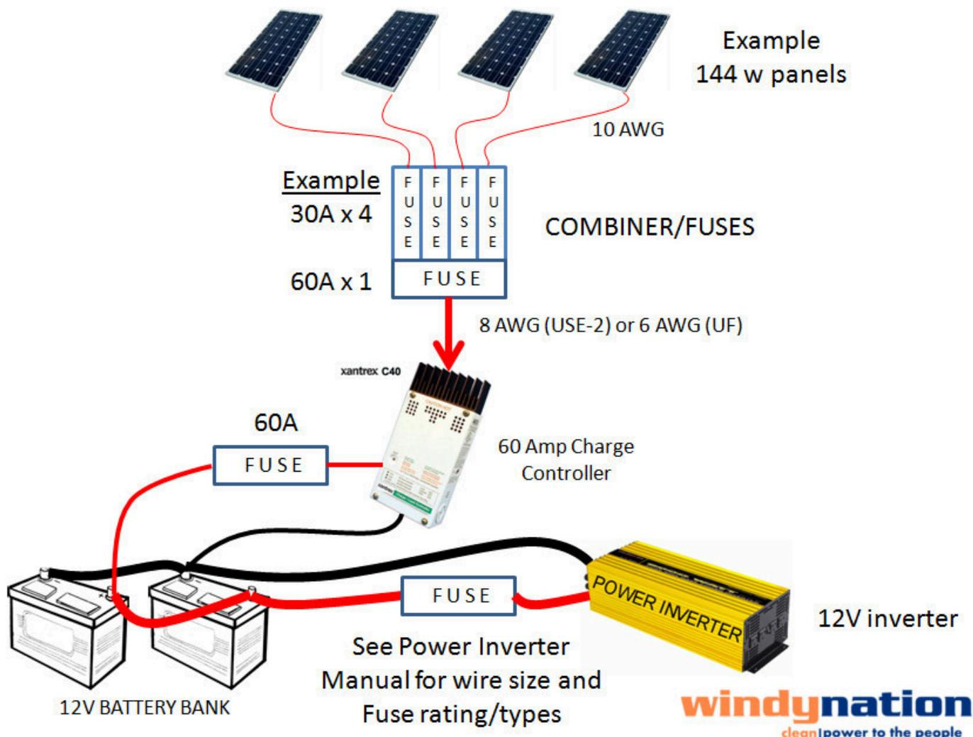
If we take the example 144-watt 12V panel from the introduction section, and look at the short circuit current ( $I_{sc}$ ), we see it is rated at 8.5 amps. This however can be exceeded if the actual installed situation does not match the "standard" test conditions used for solar panel factory ratings. The industry rule is to increase  $I_{sc}$  by 25% to cover this possibility, so it now is 10.625 amps in our example.
