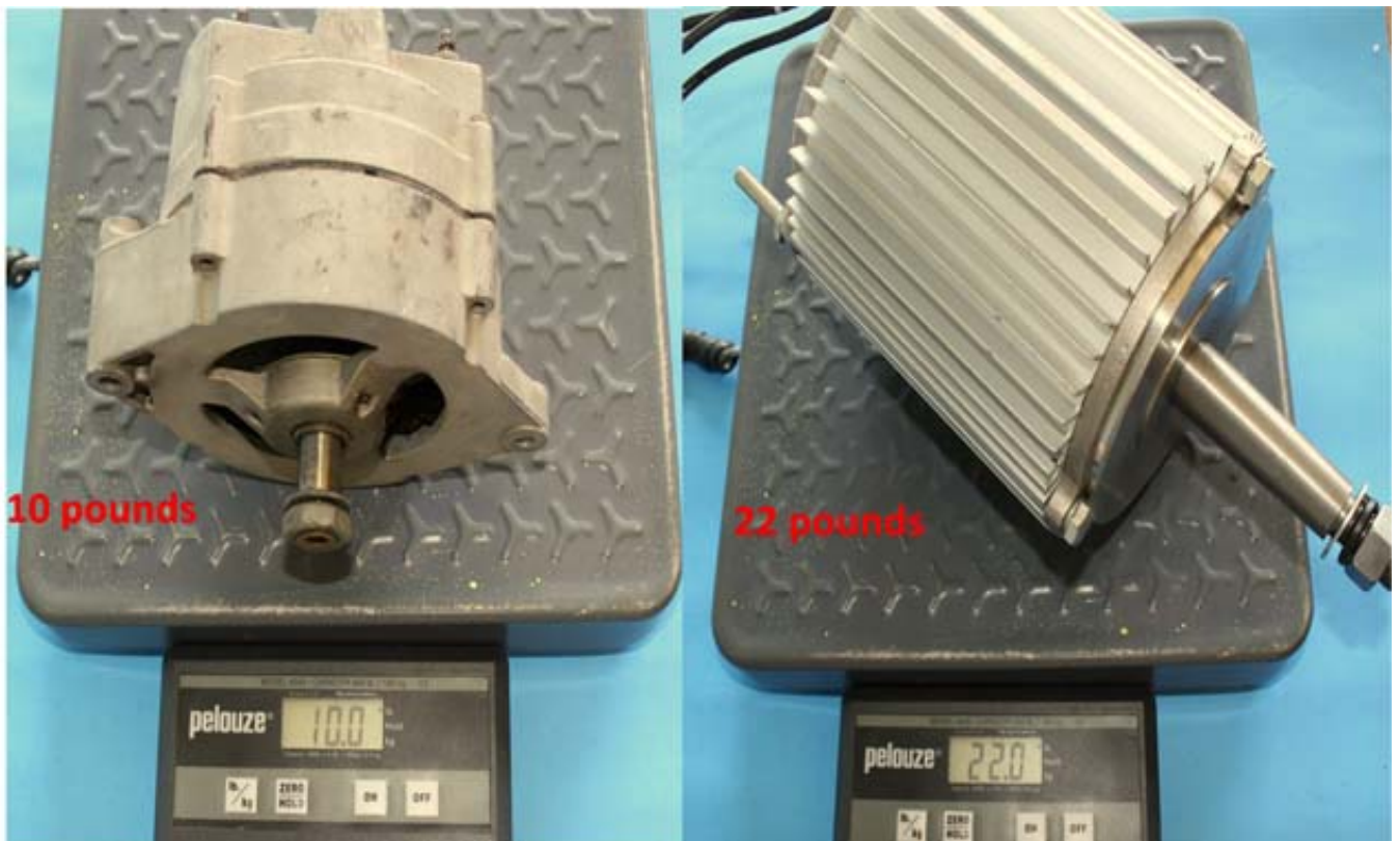
Two PMAs side-by-side on scales. The Windtura 500 (the previous generation of our Windtura 750) weighs in at 22 lbs. The Windtura 750 is about 2.5 pounds heavier than the Windtura 500.
