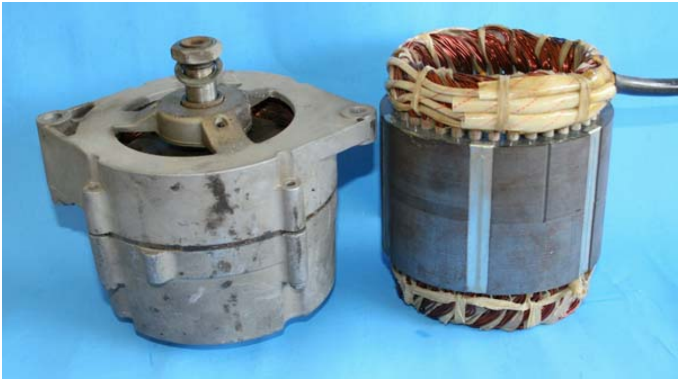
Size comparison of a Delco PMA (left) and the Windtura 750 copper stator (right).
